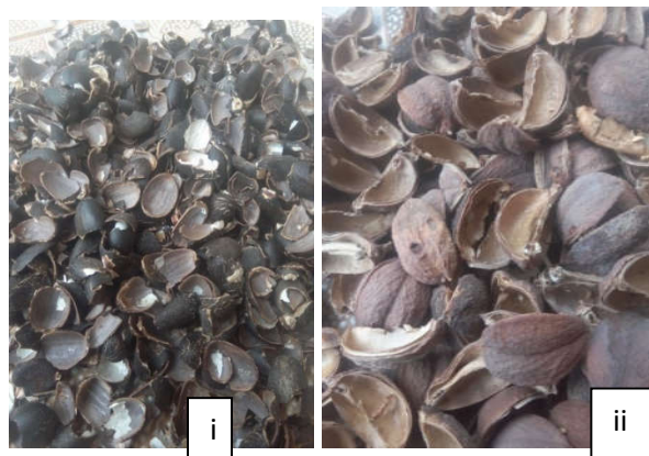
Fig 1: (i) Jatropha curcas L. seed shell (JSS) and (ii) Jatropha curcas L. fruit hull (JFH) biomasses
