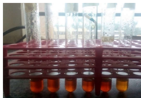
Figure 3: Carboxymethyl cellulase activity of the crude enzyme produced by Trichoderma viride under submerged fermentation
